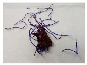
**Fig. 4** Deformation of the stent caused by extraction. During the implantation procedure, this stent migrated under the stenosis and became deformed during its extraction. Rigid endoscopic scissors and forceps had to be used
